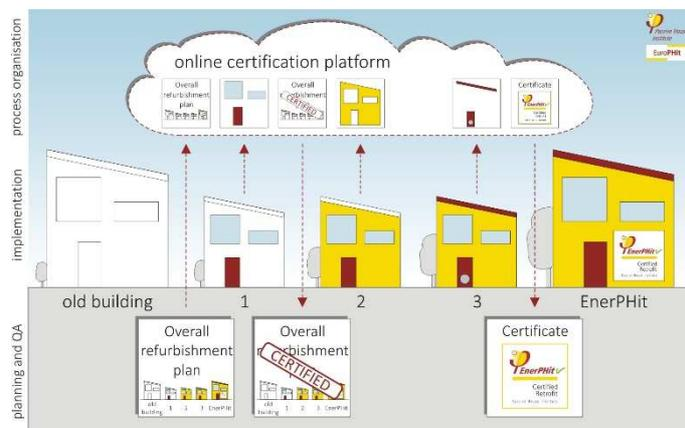
Step-by-step refurbishment focused on energy efficiency – a schematic of the concept developed within the framework of the EuroPHit project
