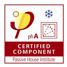
The Passive House Institute Certified Passive House Component seal for transparent building products suitable for cold climates with an efficiency class of ph A.
